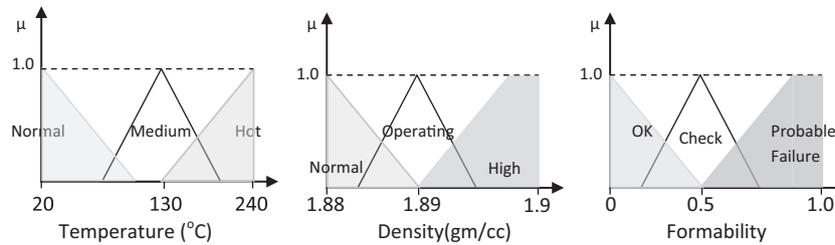
Fig. 8. Membership functions for Mg-alloy formability case study.
