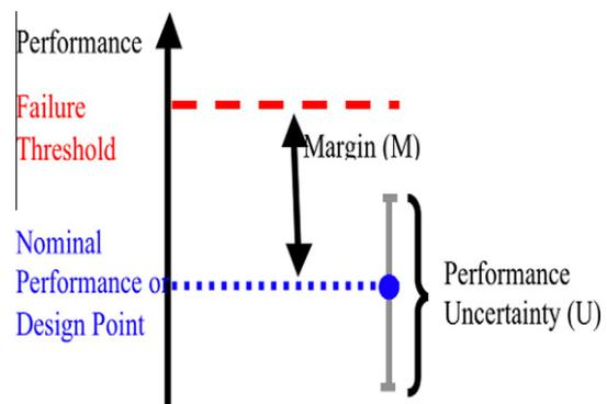
Fig. 2. QMU as defined by margin over uncertainty; this shows a threshold that is a “performance gate”.
